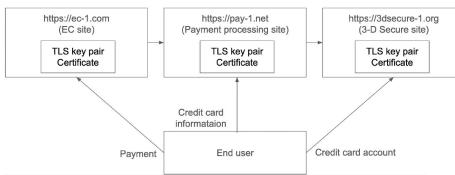
Fig. 2.1: Example environment of horizontally-chained hosts.
